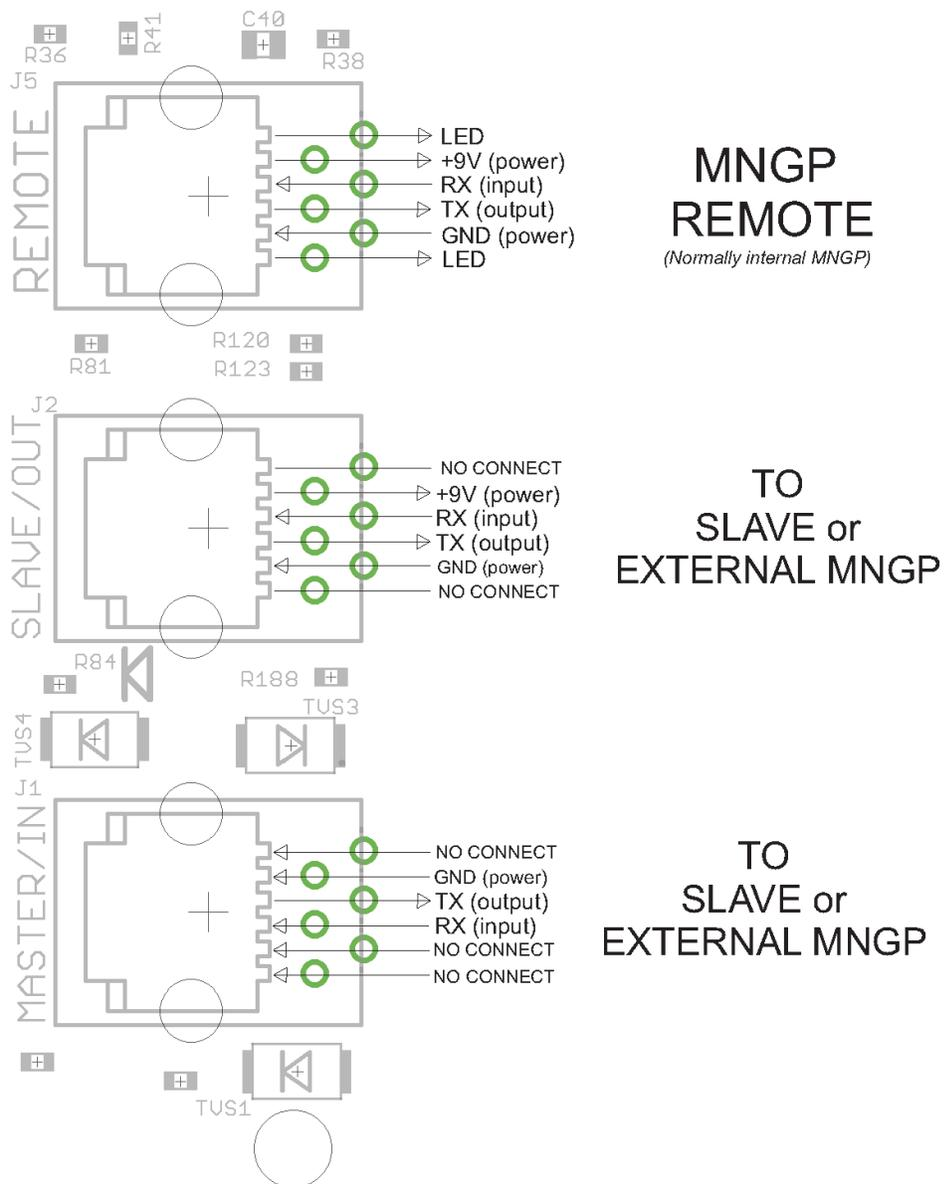
Figure 1. Classic RS-232 MODBUS RJ-11 PHONE JACK PINOUTS
