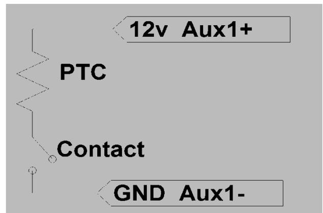
When Aux 1 is used to supply 12v out, JP6 and JP8 have to be in the position shown in Figure 3.1. The basic schematic of how this works is shown in Figure 3.2. The 12v out is more like 14.5v. The maximum current from Aux 1 should not exceed 200mA. The Aux 1 output can be set to operate at either Active High (12V) or Active Low (0V) when the Aux 1 function condition is true. For more information see [Configuring Auxiliary Input/Output](#) on page [36](#)
