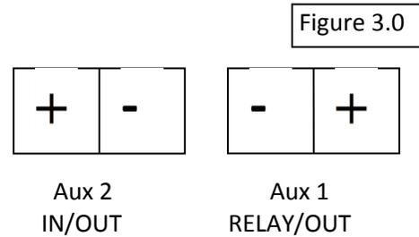
In order to select operation of Aux 1 between relay contact or 12v output JP6 and JP8 need to be configured accordingly following the instructions provided in this section.
